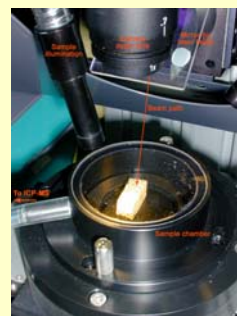
View of the sample chamber of a laser ablation probe.
